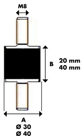
*Made of vulcanized natural rubber, they permit to insulate, control and often eliminate vibrations from external unit. Kit composed by 4 dampers with washers and nuts.*
