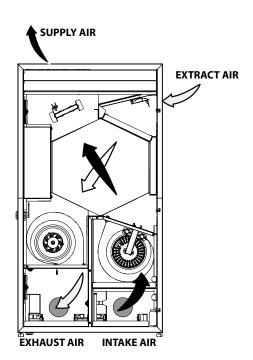
Warm stale extract air from the room flows to the unit, where it is filtered by the extract filter, then air flows through the heat exchanger and is exhausted outside by the extract fan.
