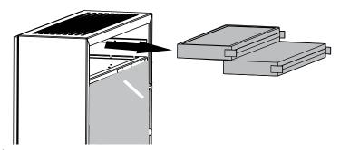
If an extract spigot is installed, remove the top protective panel and install the magnetic plug on the exhaust grille.
