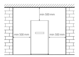
A mounting template is included in the delivery set. Fix the mounting template at the required level on the wall. Make marks to drill holes for air ducts, unit mounting and power cable entry.
