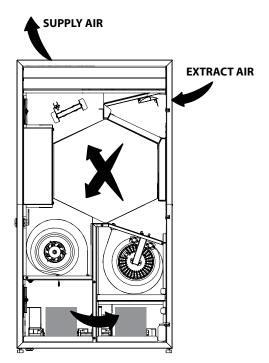
The unit is equipped with a recirculation damper. In recirculation mode it is opened and the supply and exhaust dampers are closed.
