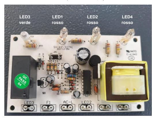
It is possible following the led signal to verify the correct functionality.
